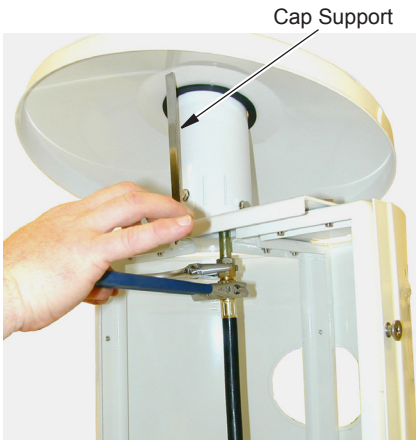
Figure 13 - Attaching Regulator and Hose Assembly
